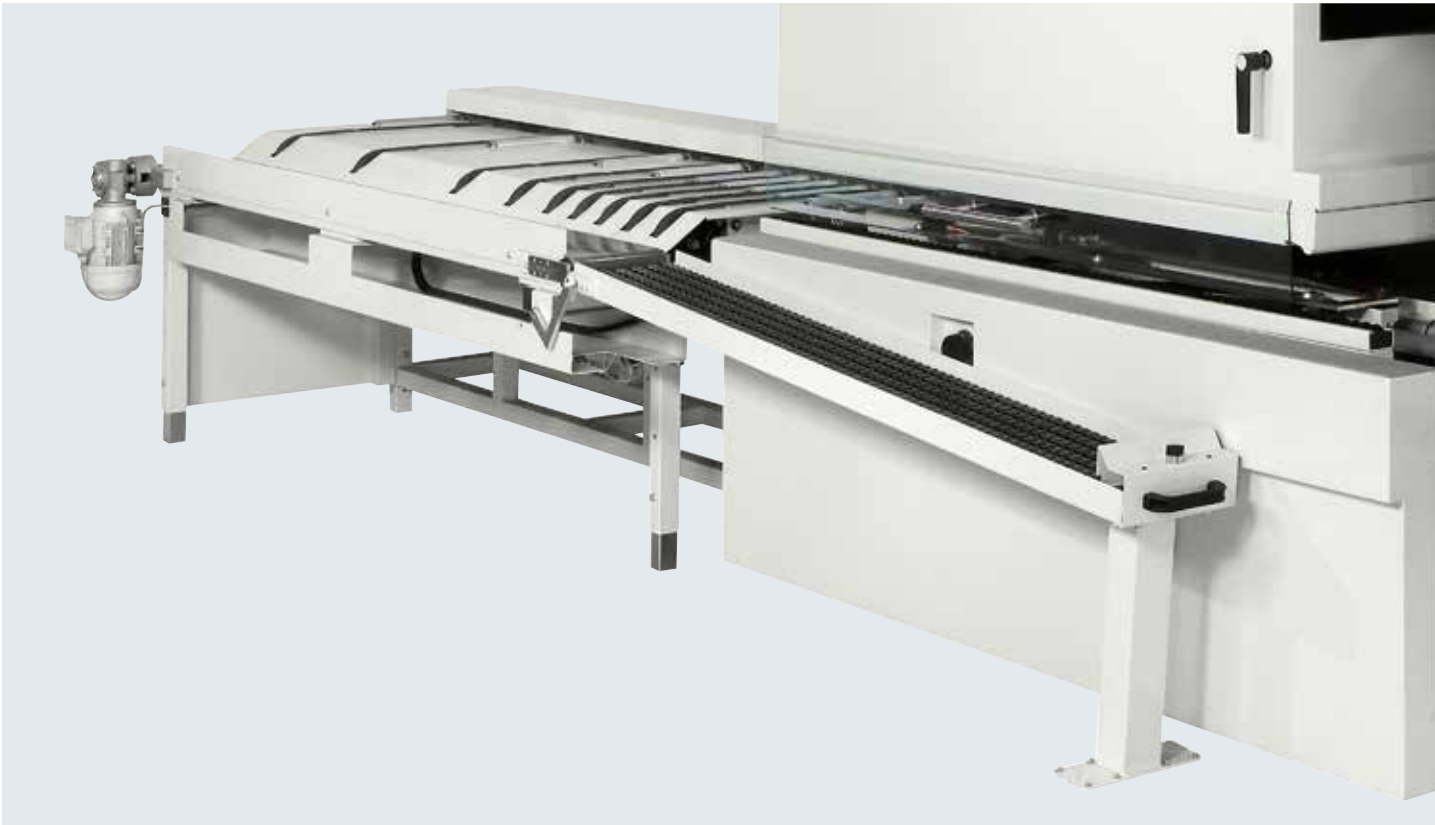
No idle time with the work-pieces return system, located at the end of the machine.
