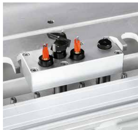
Groups for hinges For increased versatility, the quick change chucks can be fitted with various types of bits for different operations, like drilling hinges locations.
