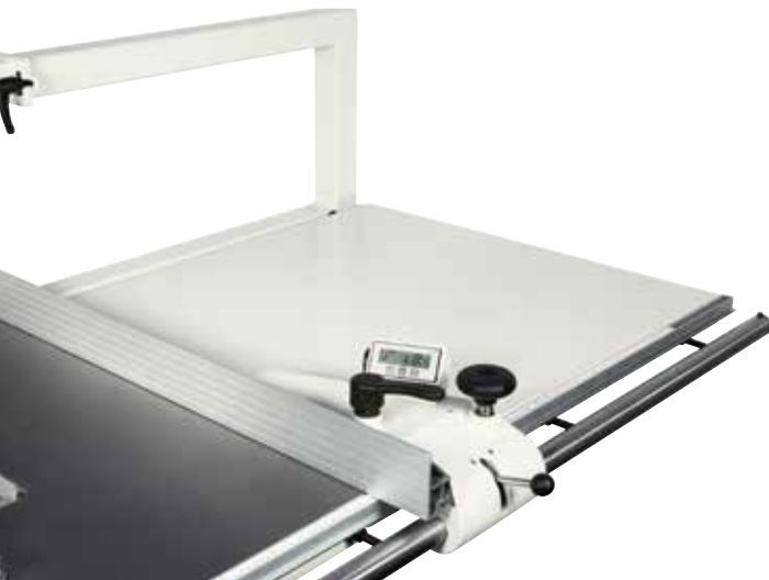
digital readout for the fence position on the parallel fence It allows precise positioning with the magnetic strip sensor.
