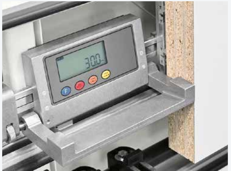
Digital vertical measuring display
