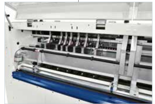
Longitudinal cutting and creasing units
