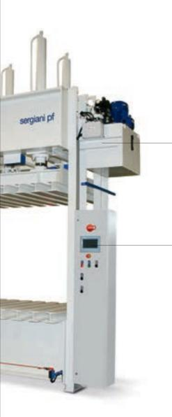
Hydraulic unit consists of a double pump and related electric motor dipped in hydraulic oil for a longer life and lower levels of noise. Automatic pressure loss recovery device ensures keeping the level set by the operator, in case of machined material failure.
