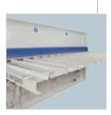
Unloading table made of steel triangle rods.
