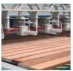
Automatic beams loading inside the press, available versions with automatic composition of panels.
