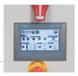
Electronic control of all machine functions via digital operator control panel with Siemens touch screen.
