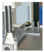
Auxiliary cylinders to control platens opening, they allow a constant and fast cycle.
