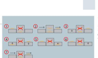
Up to 3 trays to increase productivity. While tray n° 2 is inside the press daylight, tray n° 1 is in the loading area. The third tray, once unloaded, stays underneath the press body waiting for the loading area to be released to start a new production cycle.
