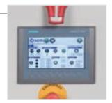
Control panel with siemens colour touch screen The control panel is equipped with a software that allows to automatically calculate the hydraulic pressure, manage the heating system, carry out a complete diagnostic, program and save all working parameters. (optional)
