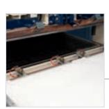
The bottom mobile platen is milled to realize all the circuits that allow creating vacuum.
