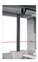
Double rack and pinion system connected by a torsion bar to grant a planar movement of the movable press platen.
